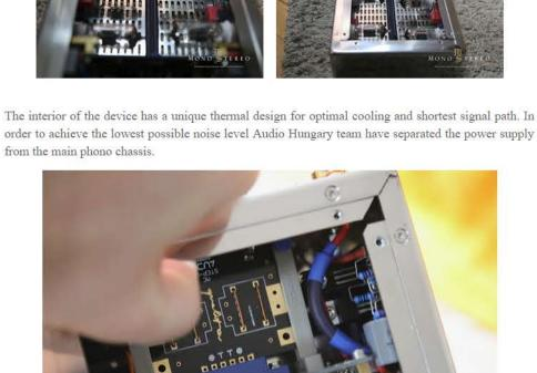
With outboard, separated power supply Audio Hungary managed to avoid the negative effects of power supply transformer magnetic field. Along the design process they discover significant benefits with
